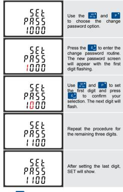
Press [\_\_\_\_\_\_ to exit the number setting routine and return to the Set-up menu. SET will be removed
