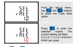
Use public and buttons to choose pulse rate. On completion of the entry procedure, press [ to confirm the setting and press [V/A] to return to the main set up menu.
