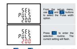
Use PF Hz and P buttons to choose pulse width. On completion of the entry procedure press [] to confirm the setting and press MA to return to the main set up menu.
