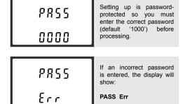
To exit setting-up mode, press MA repeatedly until the measurement screen is restored.
