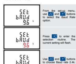
On completion of the entry procedure, press [5] to confirm the setting and press MA to return to the main set up menu.
