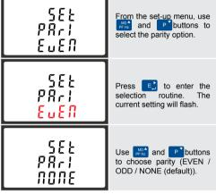
On completion of the entry procedure, press confirm the setting and press  $^{\text{MA}}$  to return to the main
