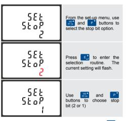
On completion of the entry procedure, press  $\[ \]$  to confirm the setting and press  $\[ \]$  to return to the main set up menu.
