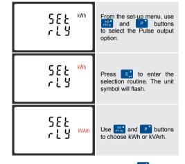
On completion of the entry procedure, press [1] to confirm the setting and press was to return to the main set up menu.
