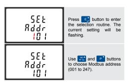
On completion of the entry procedure, press  $\begin{tabular}{c} \end{tabular}$  button to confirm the setting and press  $\begin{tabular}{c} \end{tabular}$  button to return the main
